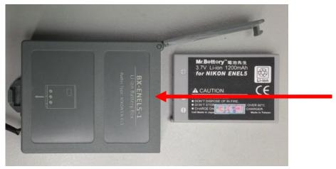
B. Install BX-ENEL5-1 battery box and GT-530 (or other device that need the battery) on DIN Rail, and connect the connector of the battery to the slot "BAT" of GT-530.
